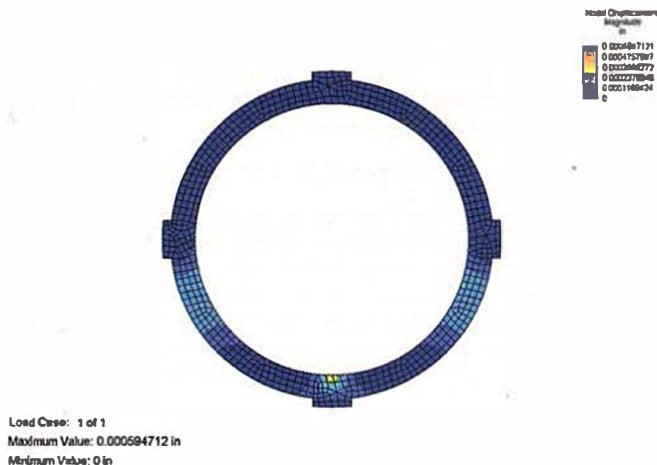
Figure 16. Displacement Result of FEA of #5 Outer Shell with LOP Configuration.
