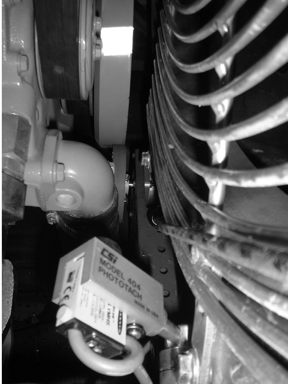
Figure 51 – Optical Encoder at Crankshaft
