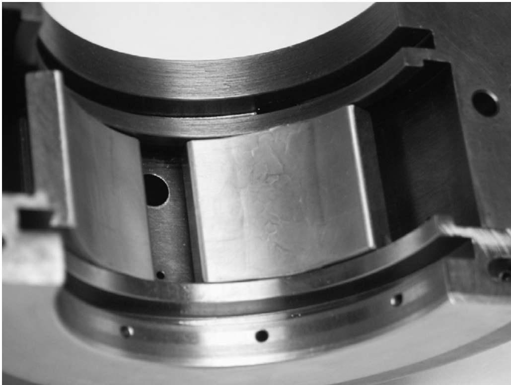
Figure 45 – Damage on Bearing Pads After Initial 20 Second Run
