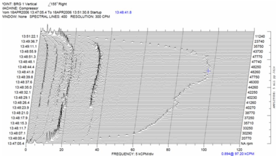
Figure 8. Waterfall of vertical probe for first full speed run of engine April 18, 2006. Turbo top speed of 97,200 rpm and dominant instability at 35,000 cpm. Keyphasor® at 1/2 so turbo speeds are 50% of actual frequency.
