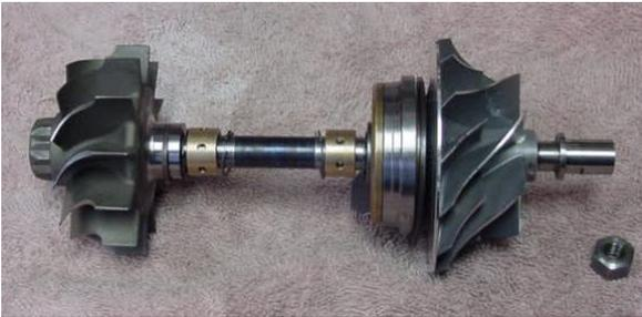
**Figure 1. A typical assembled turbocharger rotor**
