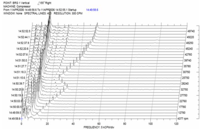
Figure 7. Waterfall plot of vertical probe for operation up to 50,200 rpm.
