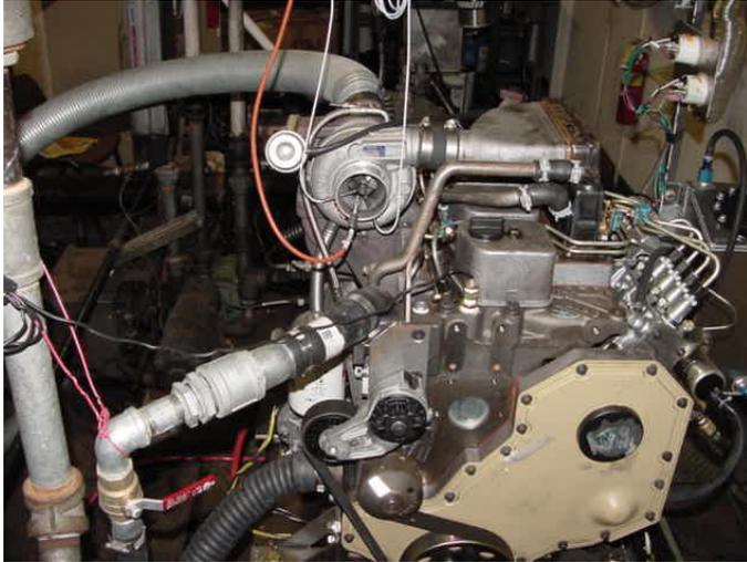
Figure 3. Diesel engine on test stand at Virginia Tech
