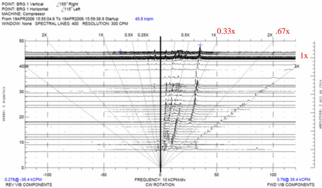
Figure 9. Cascade plot for first full load full speed run of engine April 19, 2006, Keyphasor® now at 1/3 but frequency range not adequate to show actual 1x speed when operation at full speed. Compressor shaft target nut shows same higher dominant instability at 35,400 cpm at max turbo speed.
