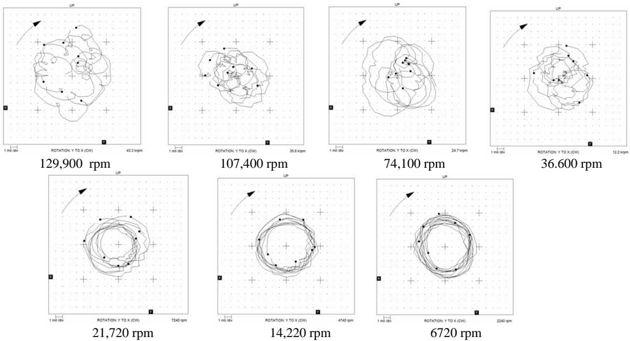
**Figure 11. Orbits for selected points of final decel of second full load, full speed run of the engine April 20, 2006.**
