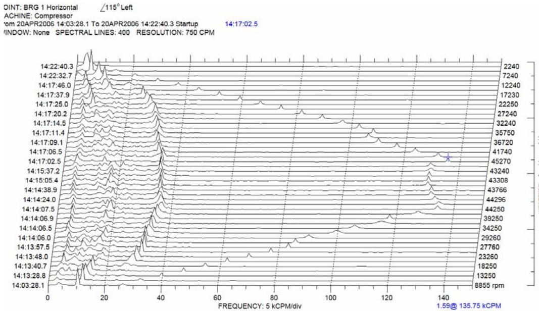
Figure 10. Cascade plot for second full load full speed run of engine April 20, 2006, Keyphasor® now at 1/3 and frequency range adequate to show actual 1x speed when operation at full speed. Compressor shaft target nut shows same higher dominant instability at near 35,000 cpm.
