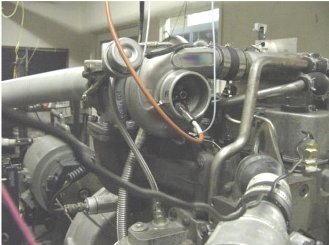
Figure 4. Compressor inlet with optical speed sensor
