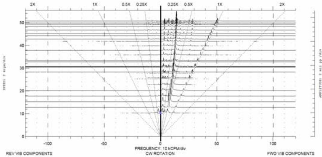
Figure 5. Cascade plot for first run of engine April 11, 2006, with turbo speed limited to less than 60,000 rpm and Keyphasor® at 1/1. Results are for compressor shaft target nut horizontal and vertical probes.
