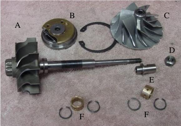
**Figure 2. Common turbcharger shaft components**
