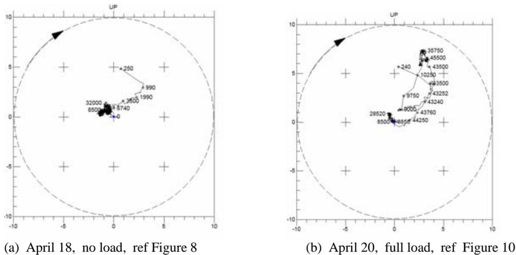
**Figure 12. Centerline plot of compressor end shaft at target nut for a) no load and b) full load. Keyphasor® at 1/3, speeds shown are 1/3 of actual shaft speed in rpm.**
